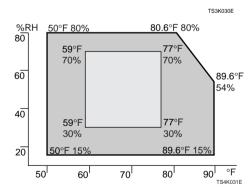
Possible operation range Recommended range The machine must be level within 5 mm, 0.2" both front to rear
